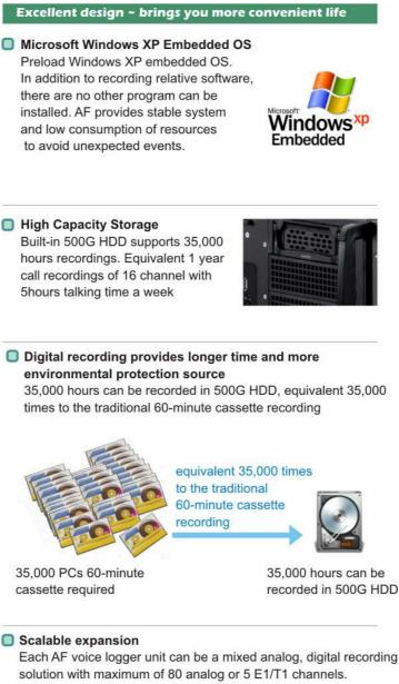
If the unit capacity is not fully occupied, number of channel can be increased simply by adding extra recording cards.
